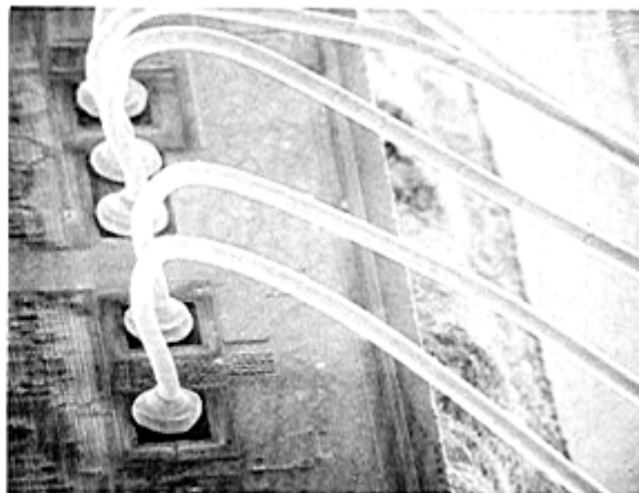
Figure 4 — The above loops were made with the reverse-motion. The loops are generally higher in profile than those made with rectangular motion. This high loop is desirable for bonding pads that are in-set from the edge of the device.
